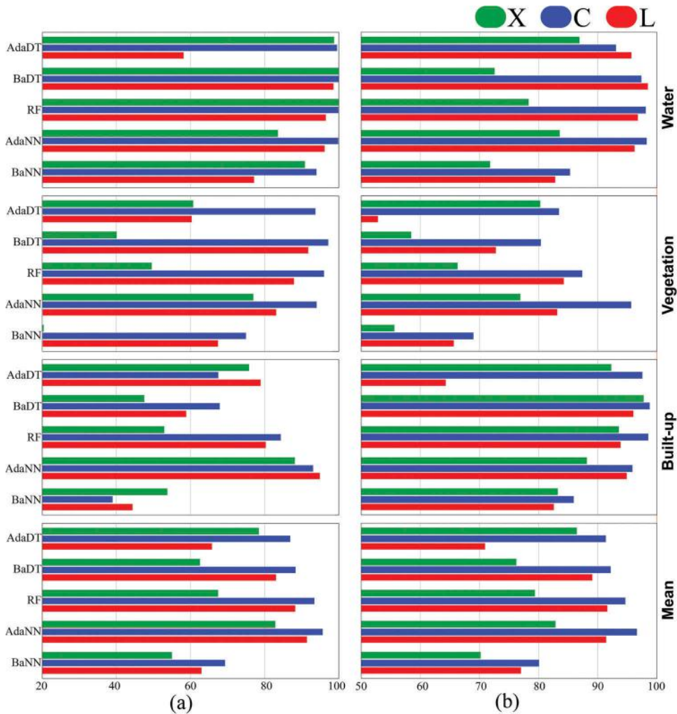
Figure 6. (a) PA and (b) UA values obtained by MCSs averaged over three training sizes in the classification of X-, C-, and L-band data sets.
