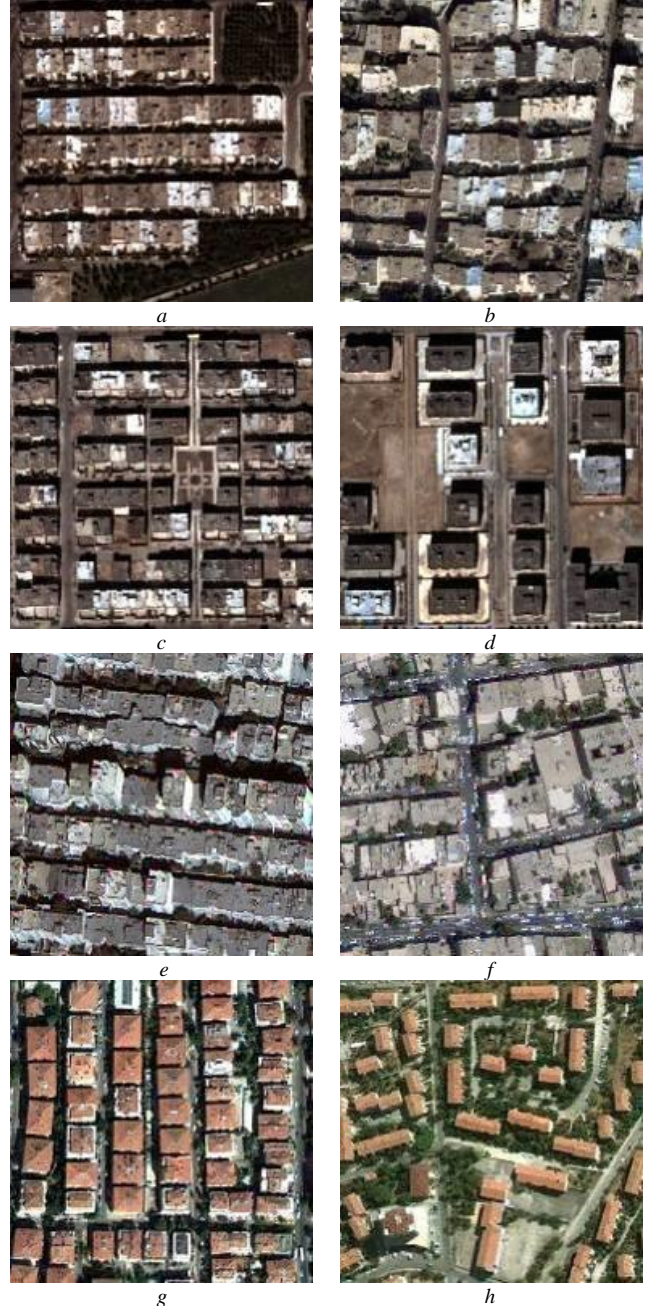
Fig. 1. (a)–(h) regions A to H. The efficient set of HSR images proposed in the paper based on challenges of urban areas focusing on building objects i.e. building density, alignment, dissociation, shape, size, color and height, in addition an oblique image.
